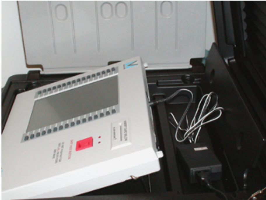
Power cord connected to the back of Infinity panel
