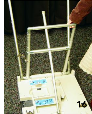
16 Collapse inner leg by depressing both sets of safety pins and pushing down.
