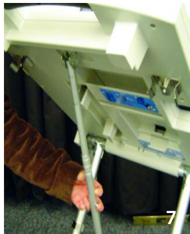
Carefully stand the unit up. To adjust the angle, lift up on the handle while pressing the safety pin on the support bar.
