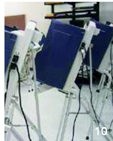
Continue plugging all the units in. The last unit will have one empty plug.
