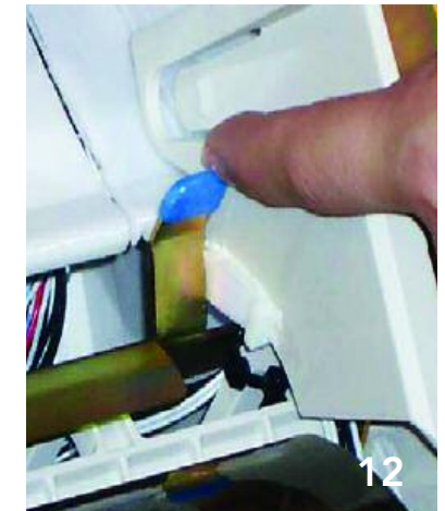
12 Unlock the AVPM by pulling the blue lever towards you. Close printer housing.
