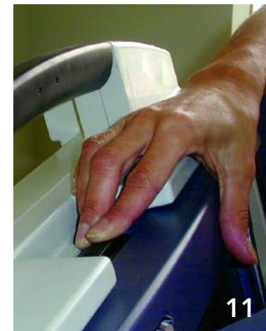
Set up one VIBS unit by pressing on the black notch while pulling the tablet forward.
