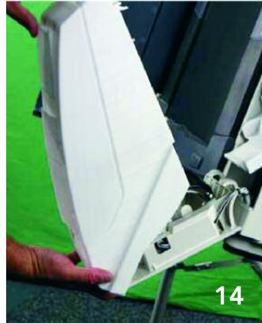
14 Gently take off the AVPM. Close the printer door and lock it.
