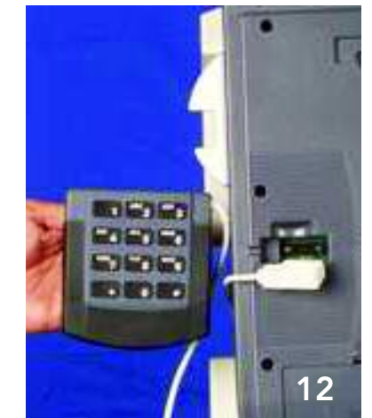
Pull the tablet out of the cradle and plug the keypad into the port on the back.
