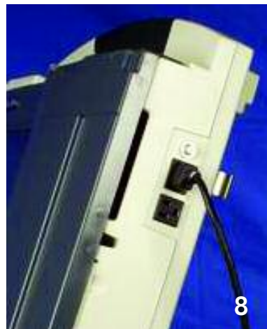
Daisy chain the units together by taking the power cord from the first unit and plugging it into an outlet.
