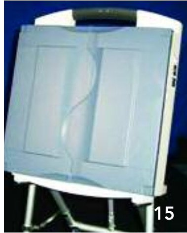
15 Close the privacy panels on the unit and seal them with a security seal. Disconnect headset, keypad and power cord from the tablet. Remove keypad from mounting slot. Close privacy screen.
