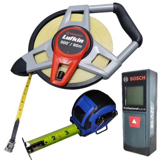
Figure 3-4 Cloth, Pocket, and Laser Tapes
