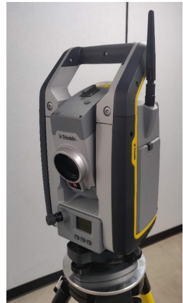
Figure 3-1 Robotic Total Station
