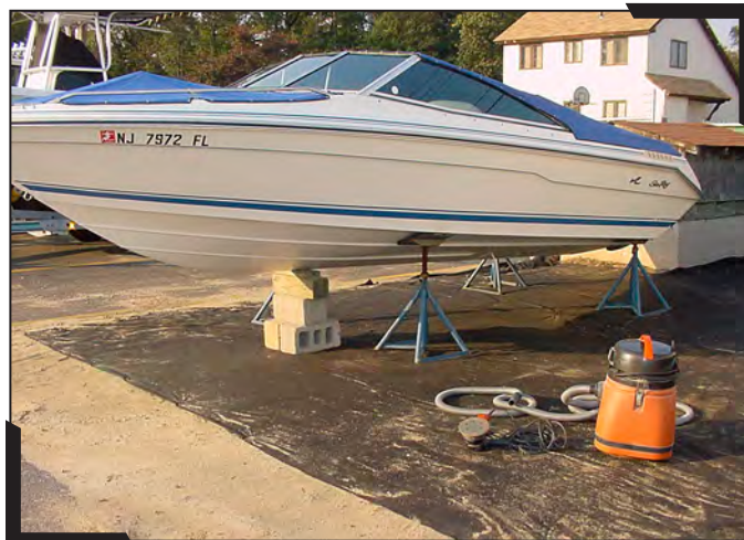
Perform boat repairs on an impervious surface over reusable permeable tarps, screens or filter cloth (Source: Jay Tanski, New York Sea Grant).
