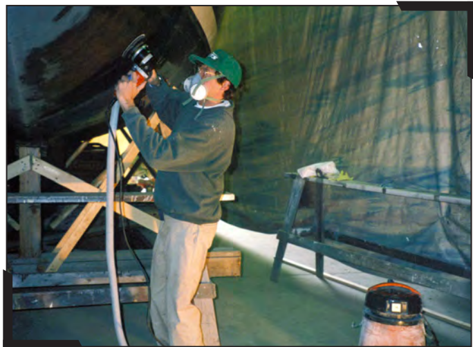
Dustless vacuum sanders are one of the best ways to control paint dust before it can become a pollutant (Source: Jay Tanski, New York Sea Grant).
