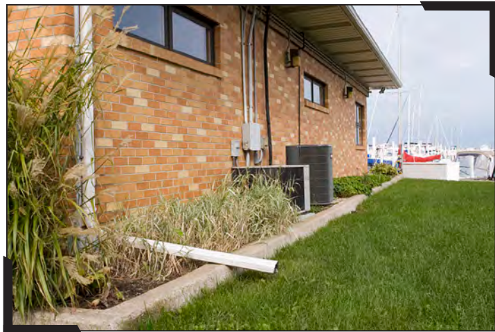
Vegetated areas can function as a buffer, filtering out pollutants between impervious surfaces and the marina basin.
