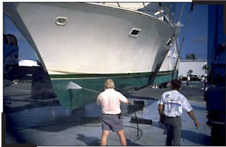
A man pressure washes a boat hull in a designated area equipped to reduce the impact of wastewater (Source: U.S. EPA Clean Marinas/Clear Value).
