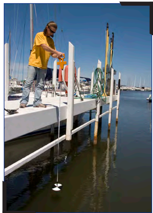
A marina employee uses a Secchi disk to measure how deep she can see into the water.
