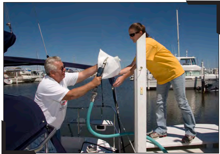
A boater and marina staff person practice spill prevention by using an absorbent cloth to prevent fuel from dripping.
