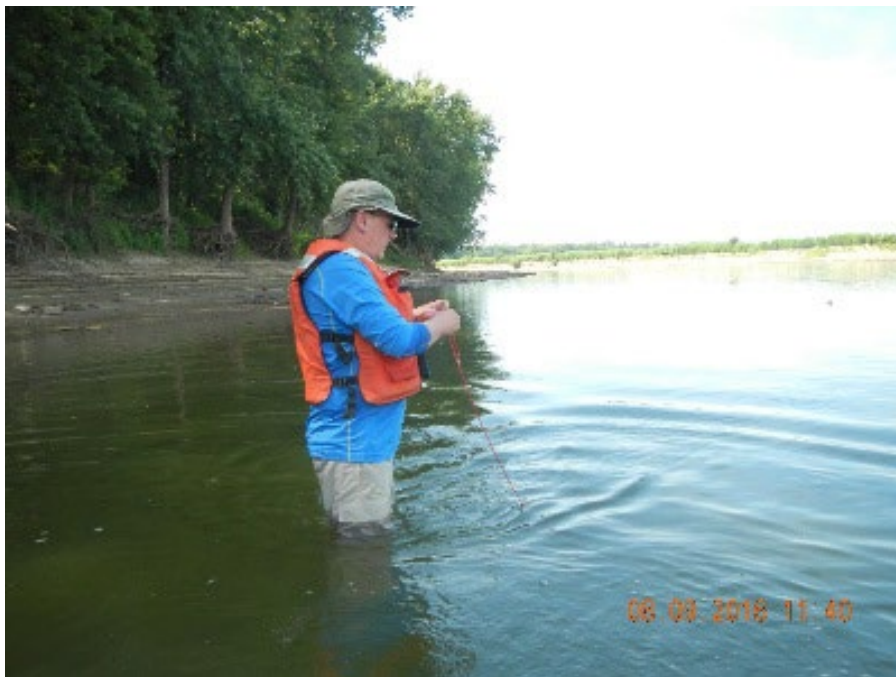
Figure 2. Attaching floats to line tied around block holding H-D samplers.
