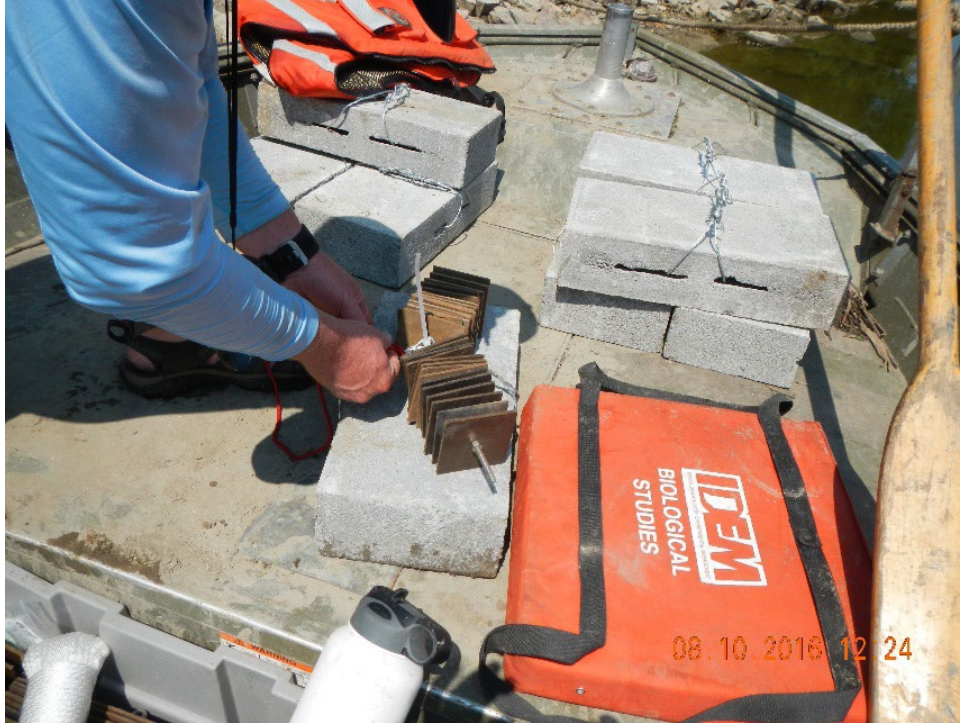
Figure 1. Attaching H-D samplers to concrete block.
