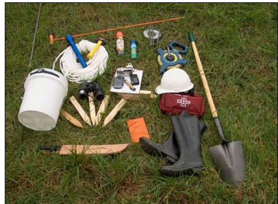
Figure 3-9 A typical inspection field kit.
