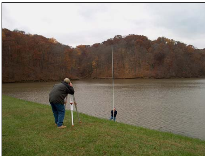
Figure 2-2 These inspectors are checking freeboard with a level and stadia rod.
