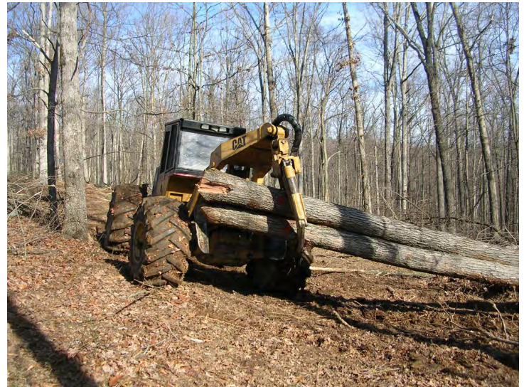
Skidder drags logs from harvest area towards log landing creating a skid trail.
