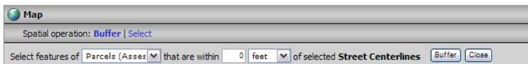
Figure 21—Spatial Selection Toolbar with the Buffer Operation Selected.
